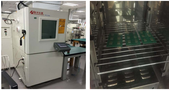
Fig. 7. Temperature chamber and test board within the chamber.
